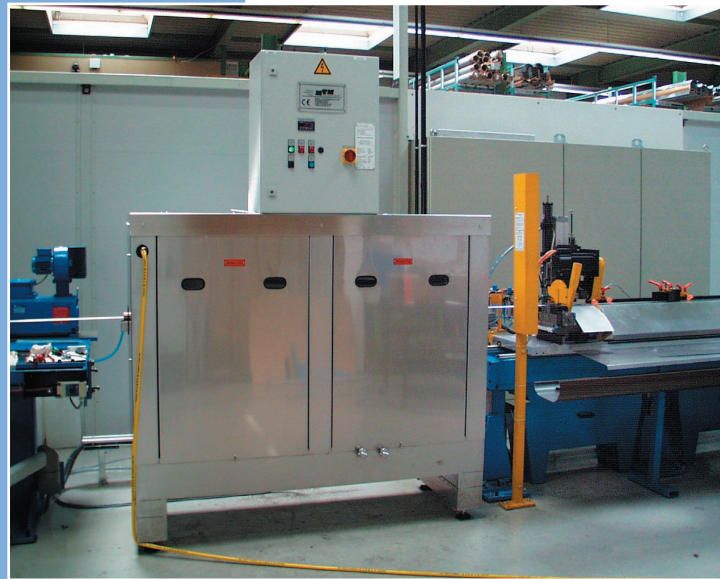
Fluting - MTM-Steam cleaning system (with switch cabinet) - filling measuring
